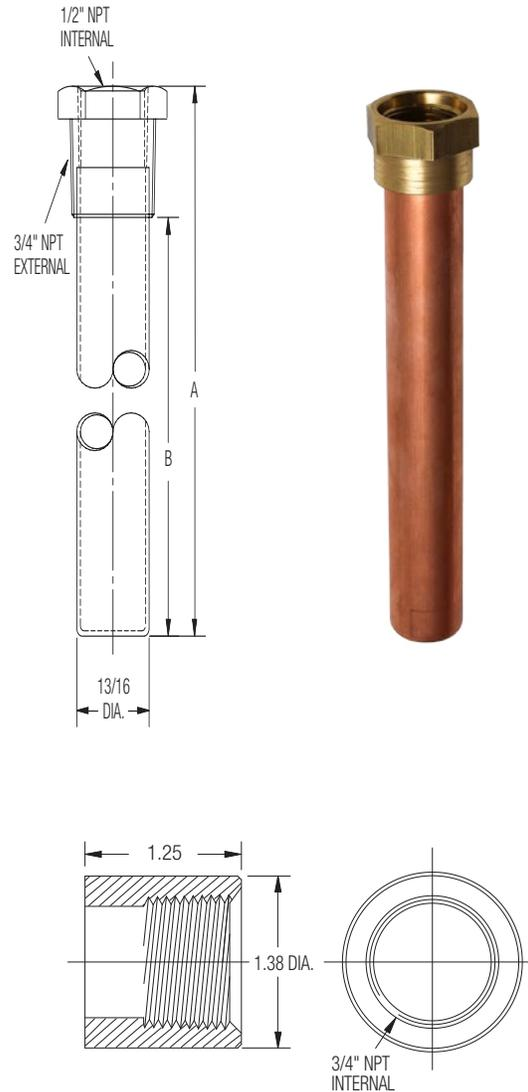
**65187 Half Coupling** - Mount to Reservoir. For use with all bulb wells shown above.
