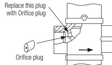
All stock valves are supplied with a drilled and tapped internal by-pass in the regulator body. A solid plug is installed in this hole for 100% shut-off. A drilled orifice plug is packed in an envelope with each valve for field installation, if continuous minimum flow is required.
